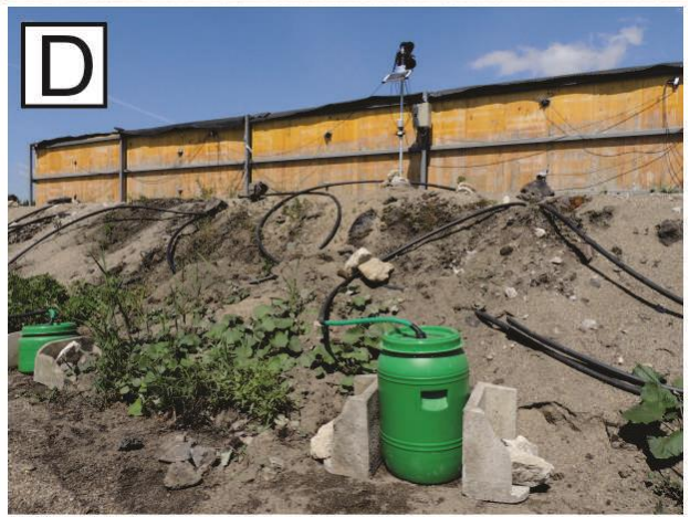
Figure S2 Different stages of a field construction of lysimeters: Metal rod support structure (A) and the same structure placed at the final location of lysimeters (B), installation of an internal box structure, made from water resistant formwork plates (C), and the bottom-up view on the finalized structure of the box lysimeters, with a lysimeter percolate collection tank placed in front (D).
